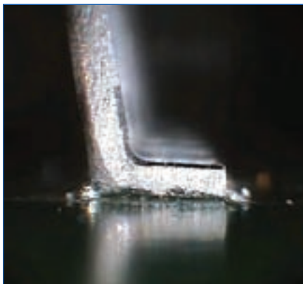
Figure 5. Lead-free joint on a gull wing lead with a tin finish.
