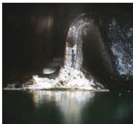
Figure 6. Lead-free joint on a SOIC after reflow soldering in a convection process.
