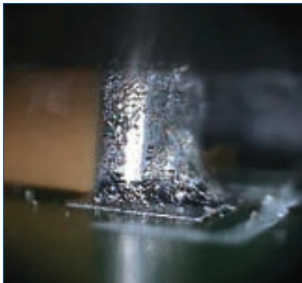
Figure 4. Chip capacitor with a tin termination soldered with tin/silver/copper lead-free paste.
