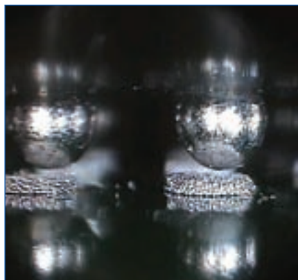
Figure 9. Another BGA package that has not been placed into the paste deposit.
