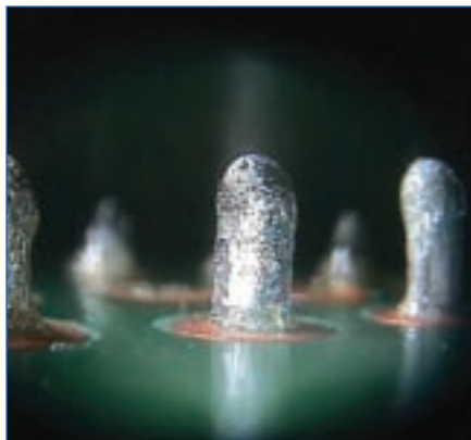
Figure 11. An incorrect profile resulted in partial reflow on the pin.
