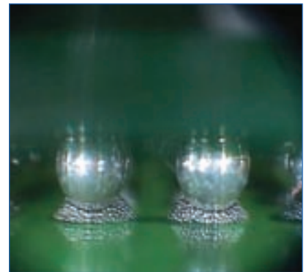
Figure 9. The balls in this part are plastic with a metallised solderable coating.
