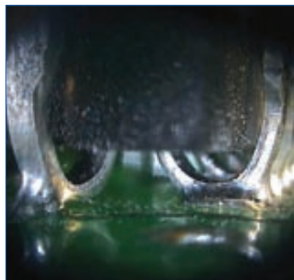
Figure 3. The joints have not formed under the body of this part.
