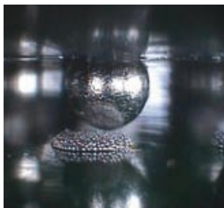
Figure 1. The BGA package has not been placed into the paste deposit.
