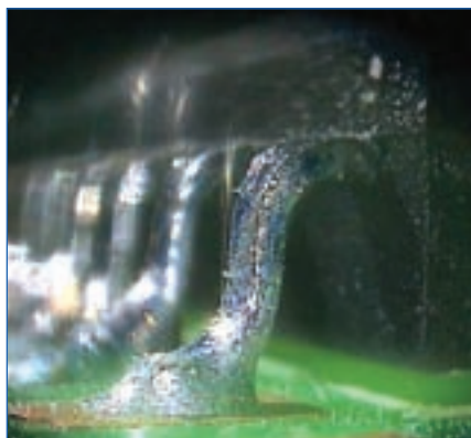
Figure 8. These lead-free joints have failed to wet correctly.
